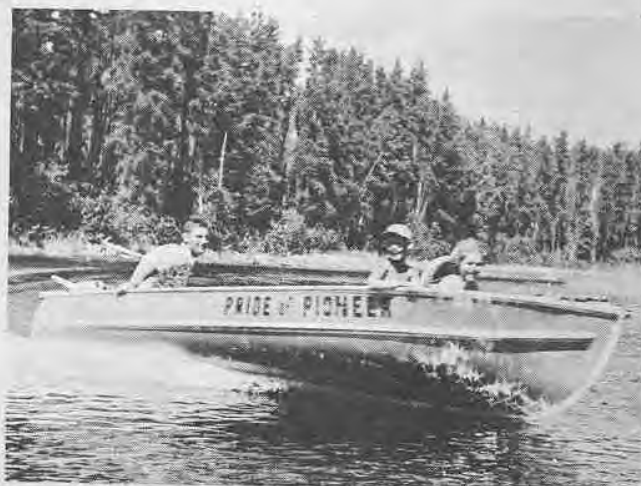
The Pride of Pioneer is one of eight models made of die-formed steel.
