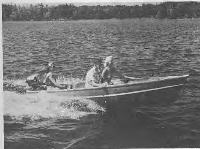
(Top) Tomahawk Car Mate has 12-foot fiberglass hull and weighs 110 lbs. (Bottom) Pere Marquette utility boat is built of laminated fiberglass.
