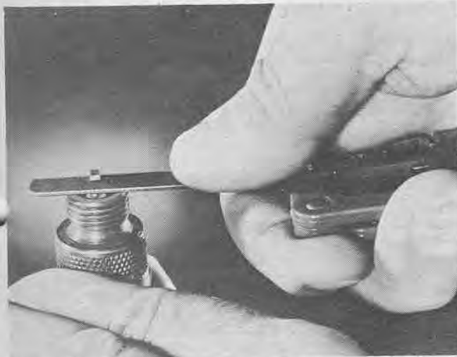
The electrode sparking areas should be faced off flat and parallel.
