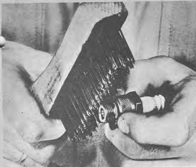
Use a petroleum solvent to remove oily fouled deposits from spark plugs. Use wire brush or rotary wire buffer to keep plug threads clean.
